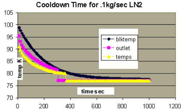
Figure 3: Model of the cooldown by LN<sub>2</sub> over 20 min of 40 K temperature rise of a 15-T magnet pulse.
