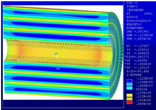
Figure 5: Axial stress during LN<sub>2</sub> cooldown.
