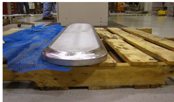
As-Constructed Obround PMCap
